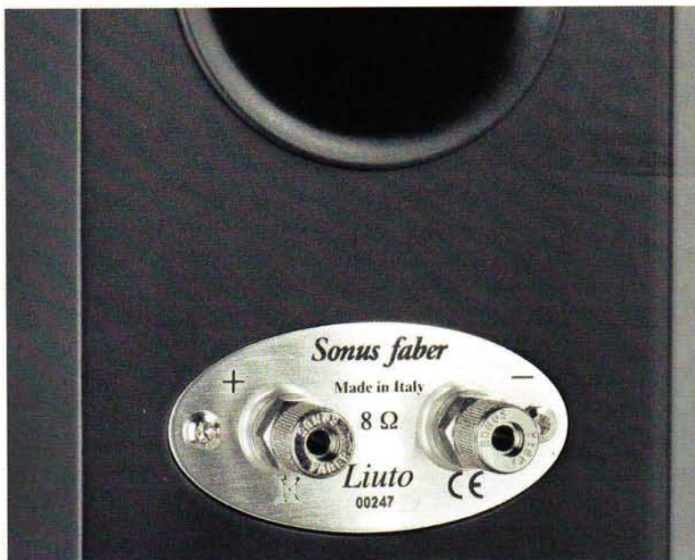
ABOVE: Presenting an easy load to the amplifier, the Liuto Tower speaker is nonetheless sensitive to room positioning and is not designed for bi-wiring/amping
